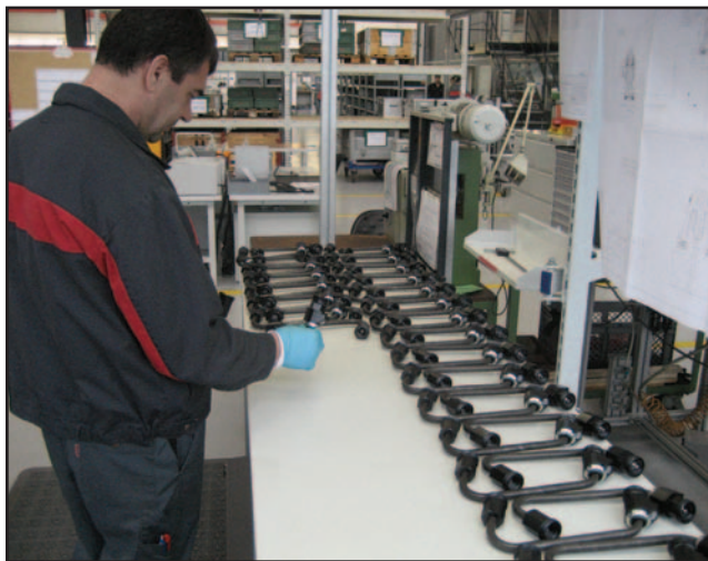
(Left) Final assembly of high-pressure piping. (Right) After flashing a high-pressure piping, the filter is submitted to microscopic examination to assess internal cleanliness.
