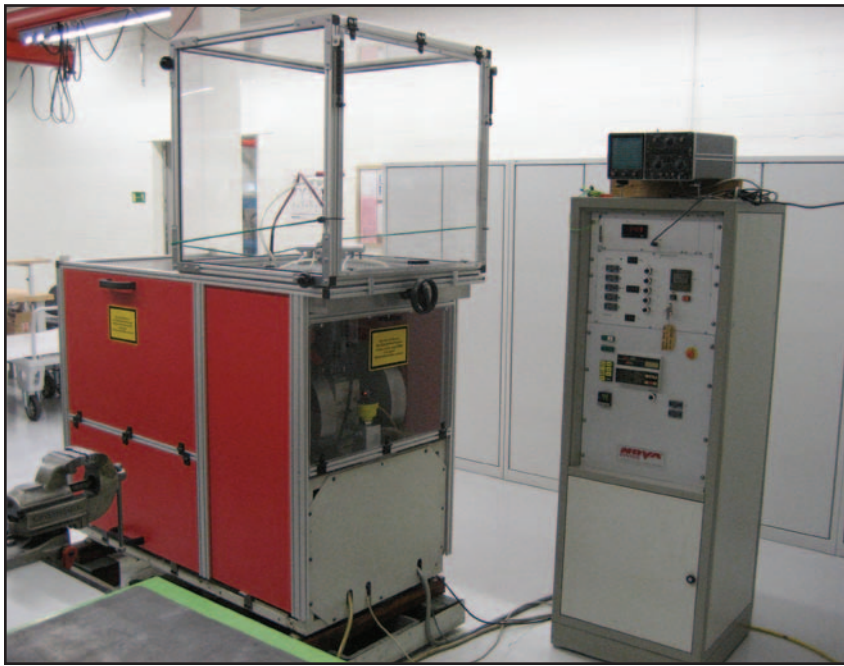
Fuel system components are submitted at 4000 bar pulsations on this test stand.
